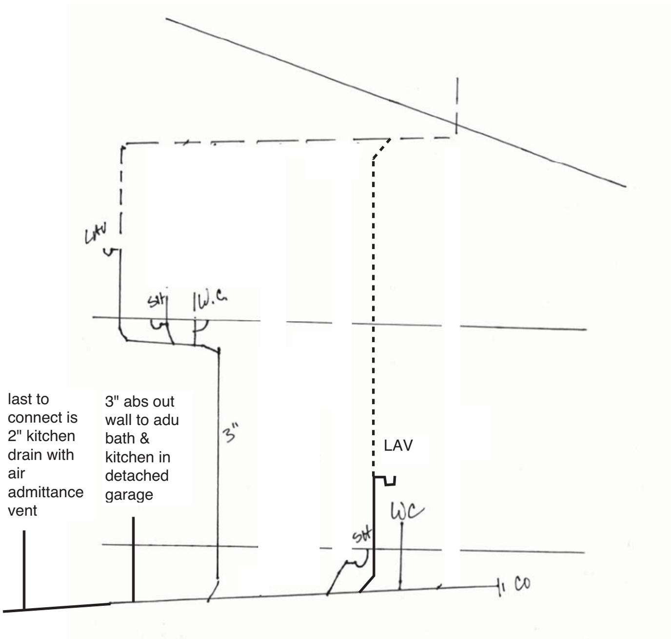
last to connect is 2" kitchen drain with air admittance vent
