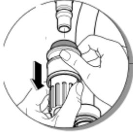
Then unthread the black end of the coupler from the hose, this should be hand tight Only, then pull the spring off.
